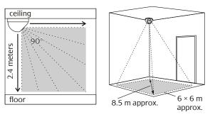
Figure 2 - The 5751L sensor's detection field
